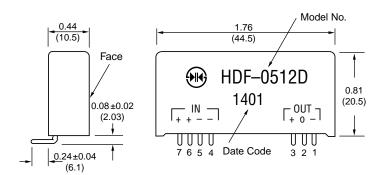
With optional formed leads available - use "-F suffix." Dimensions in inches; ( ) Dimensions in mm.
