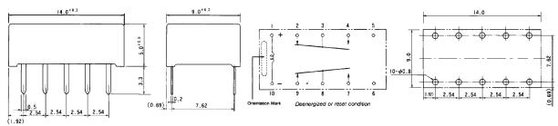
AL-D type (Double winding latching type)
